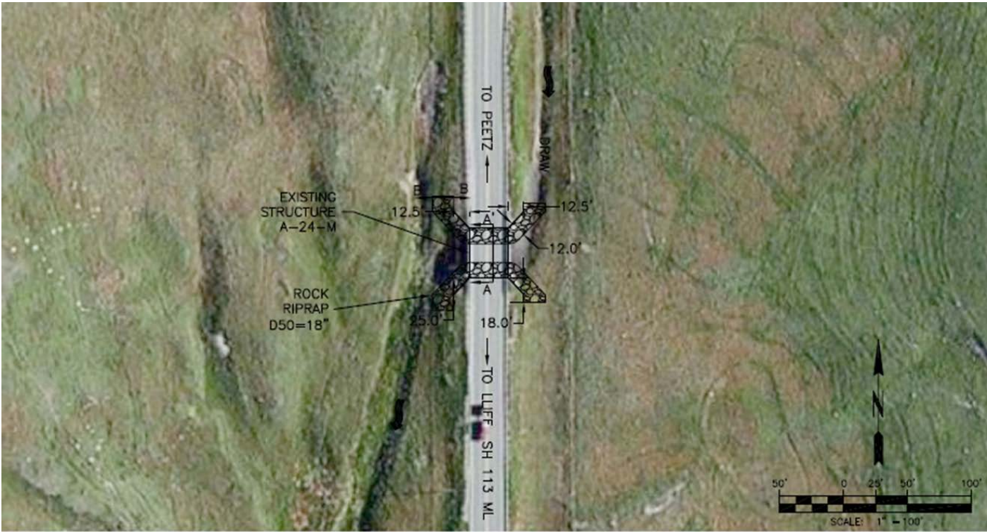
Figure 5. Plan view of Bridge A-24-M with recommended hydraulic scour countermeasure locations
