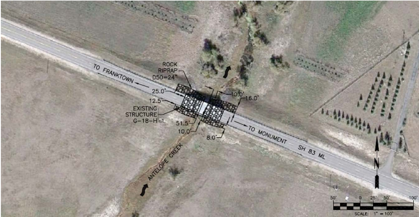
Figure 5. Plan view of Bridge G-18-H with recommended hydraulic scour countermeasure locations
