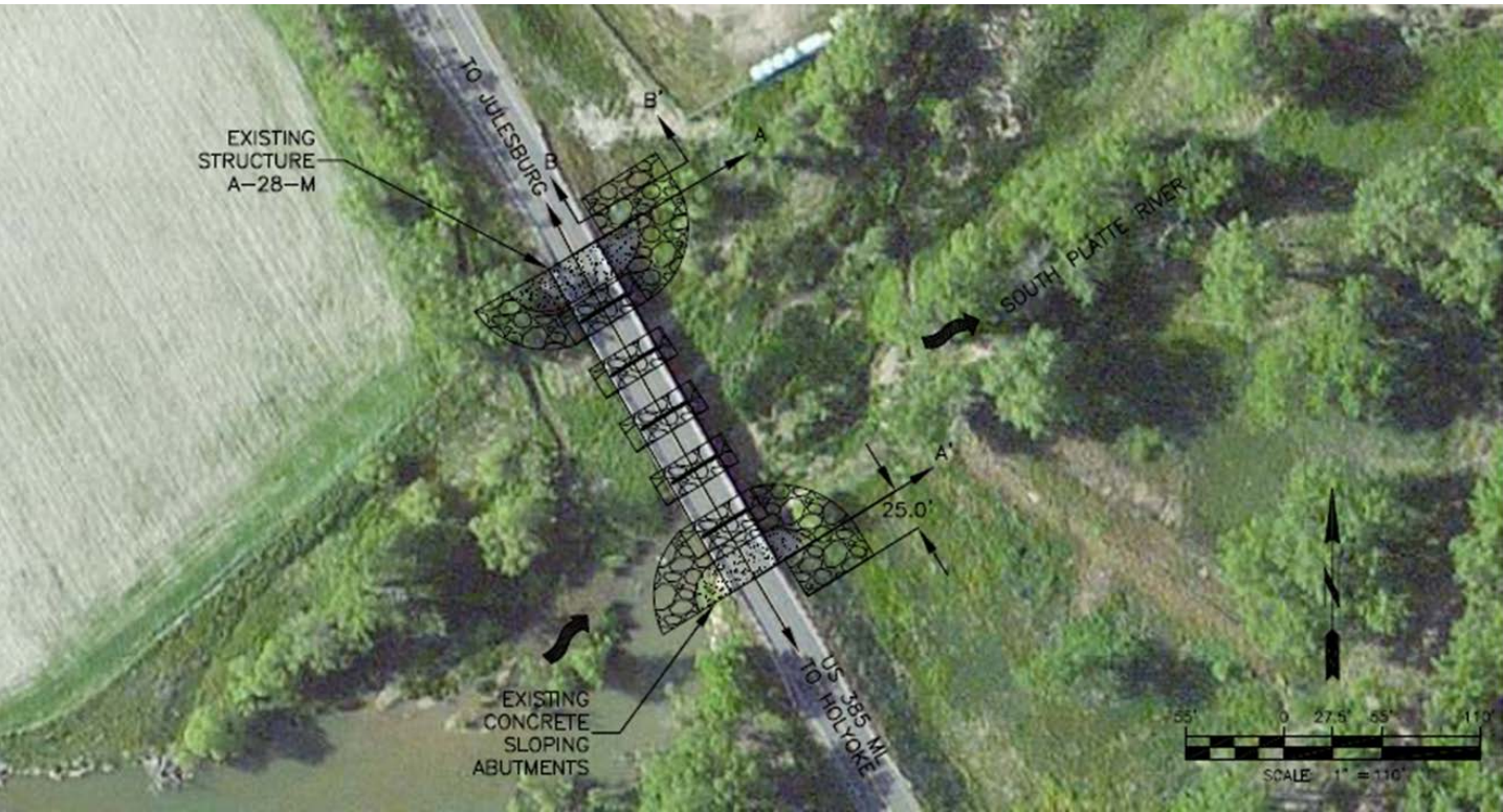
Figure 5. Plan view of Bridge A-28-M with recommended hydraulic scour countermeasure locations
