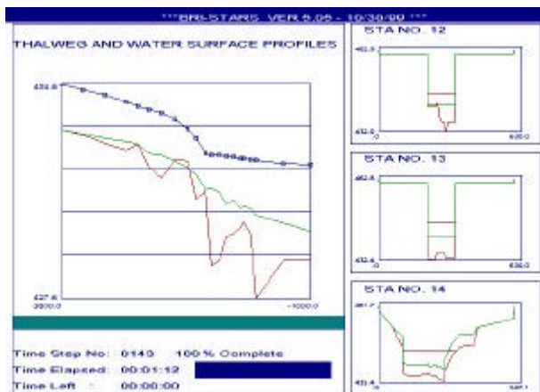
Figure 5. Thalweg and Water Surface Profiles window showing the initial (green) and final (red) ground profiles of study reach.
