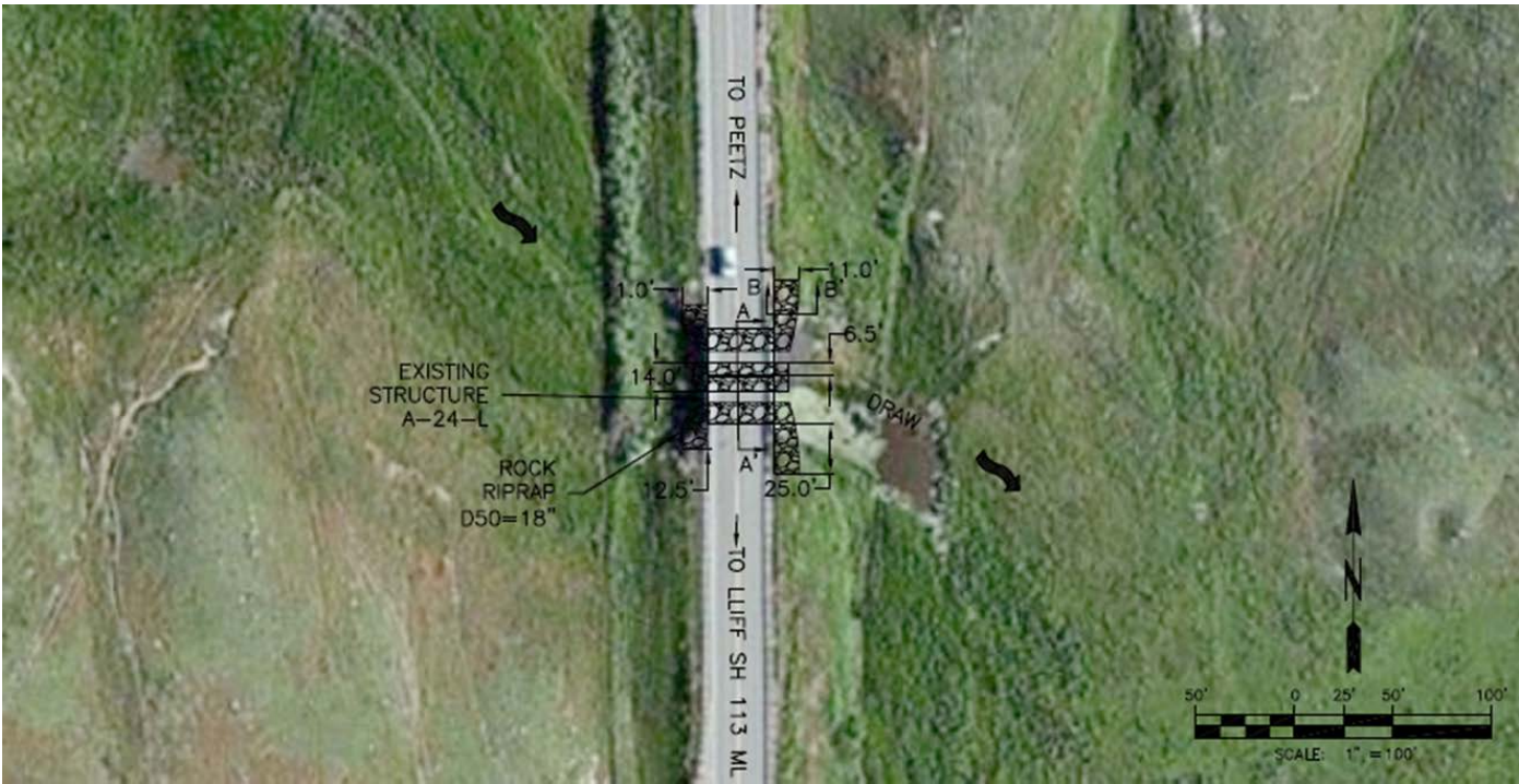
Figure 5. Plan view of Bridge A-24-L with recommended hydraulic scour countermeasure locations
