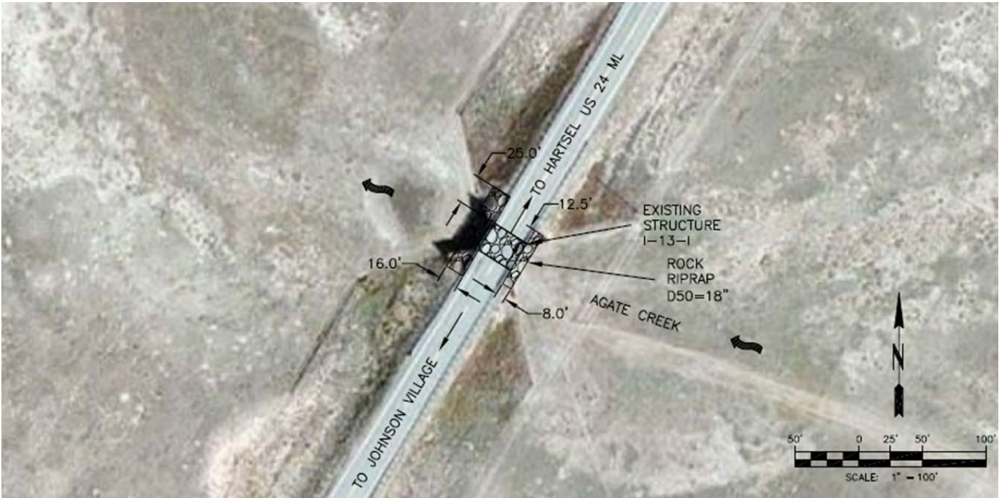
Figure 5. Plan view of Bridge I-13-I with recommended hydraulic scour countermeasure locations
