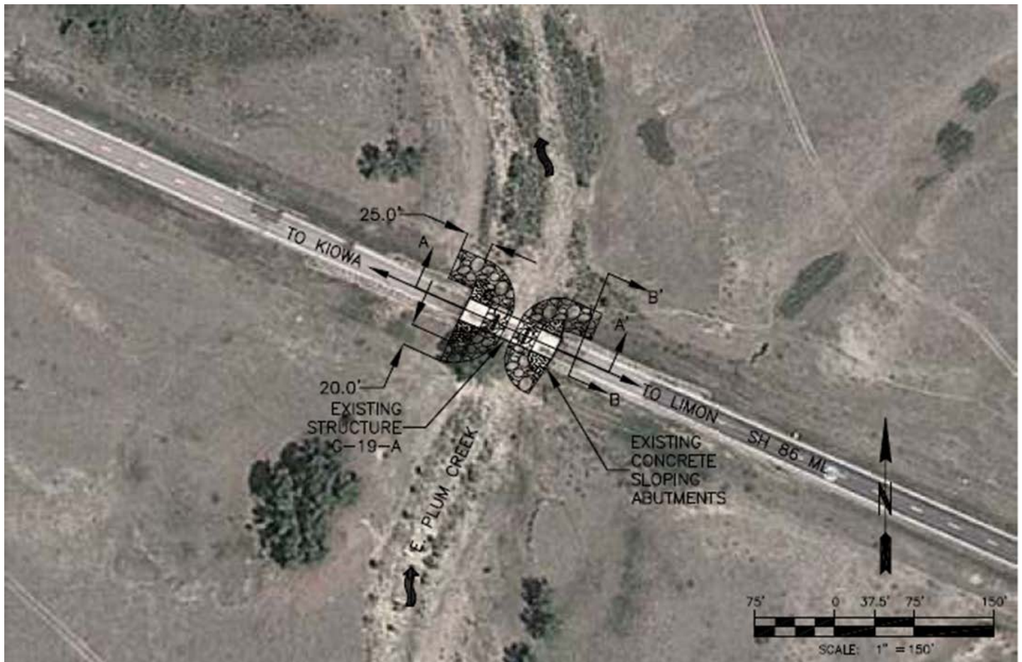
Figure 5. Plan view of Bridge G-19-A with recommended hydraulic scour countermeasure locations
