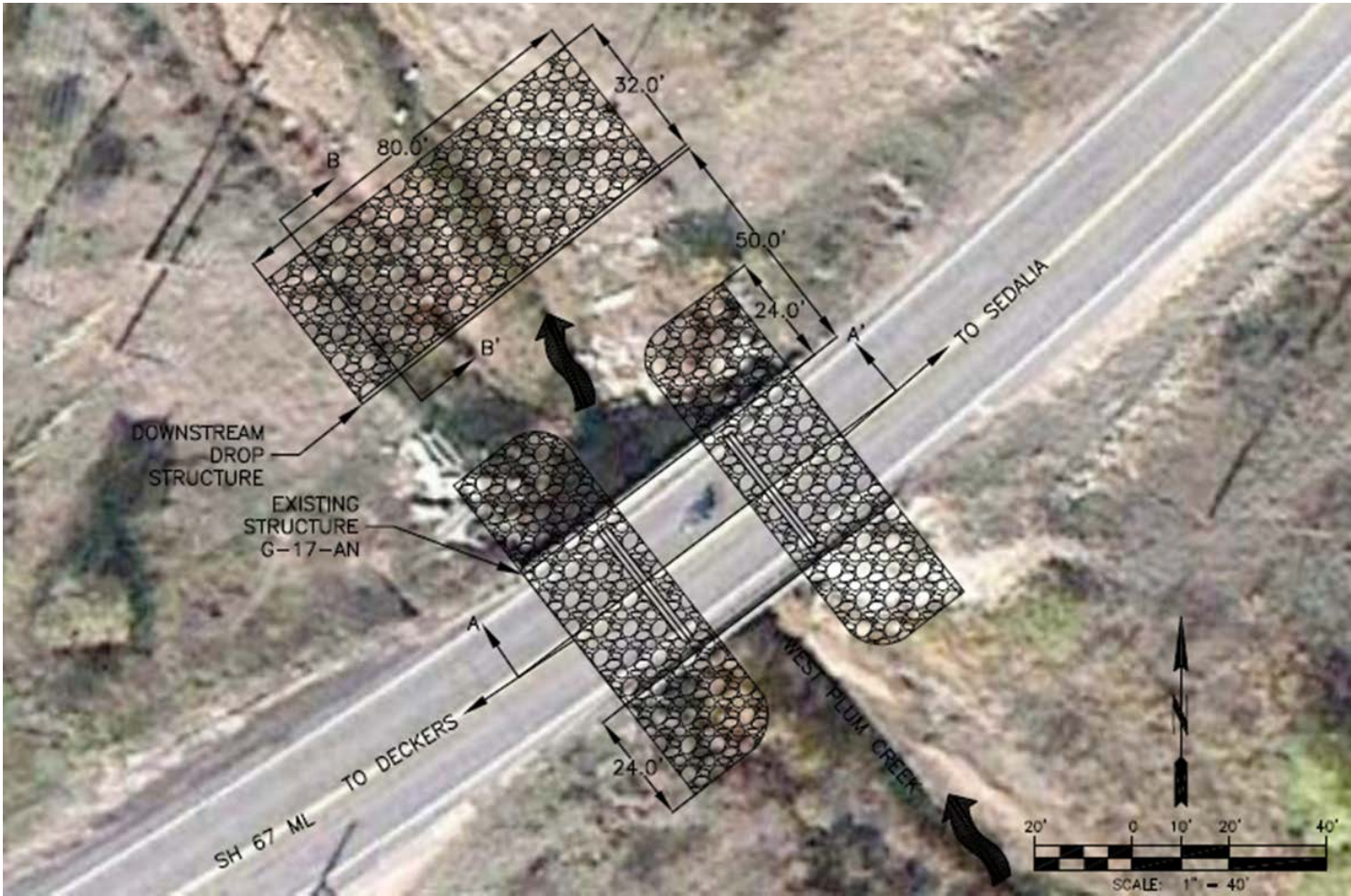
Figure 5. Plan view of Bridge G-17-AN with recommended hydraulic scour countermeasure locations
