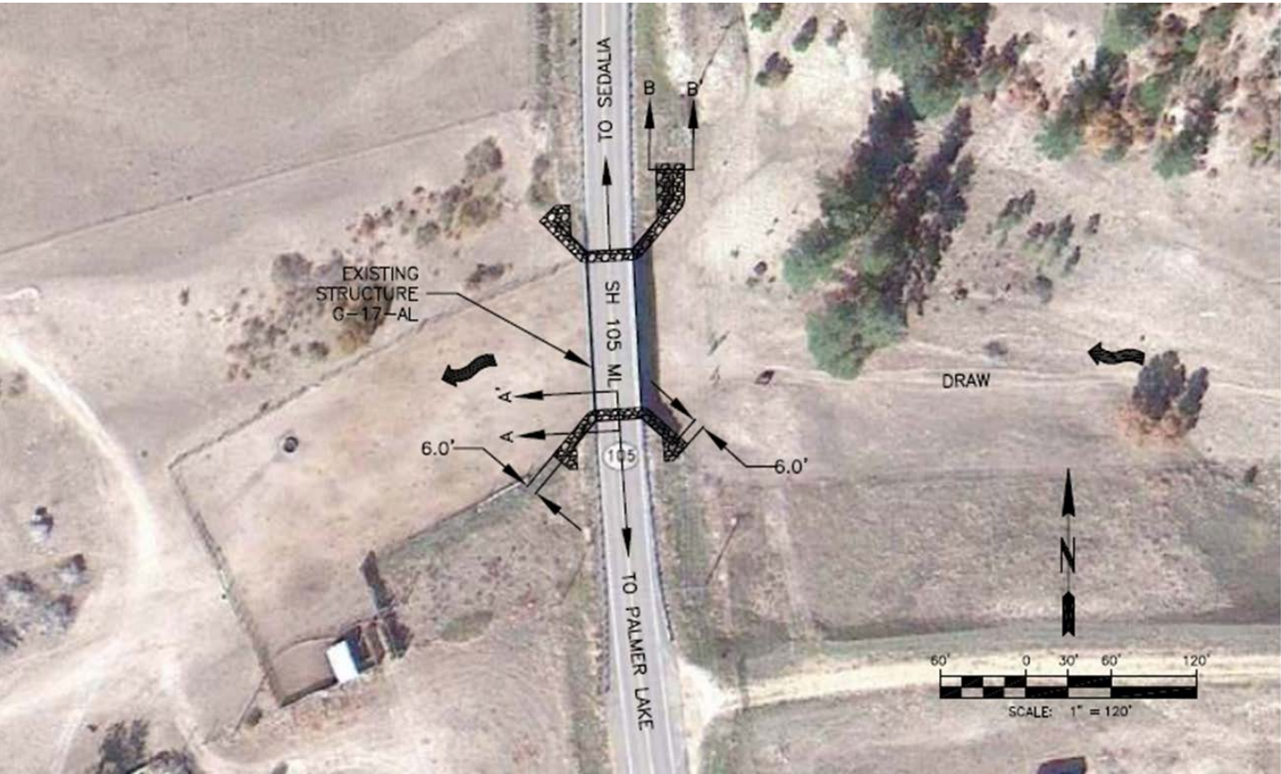
Figure 5. Plan view of Bridge G-17-AL with recommended hydraulic scour countermeasure locations
