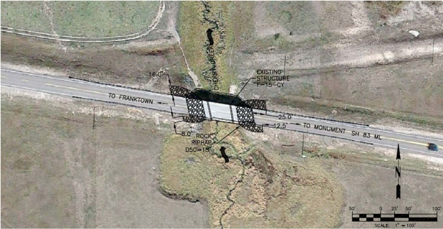
Figure 5. Plan view of Bridge G-18-BC with recommended hydraulic scour countermeasure locations
