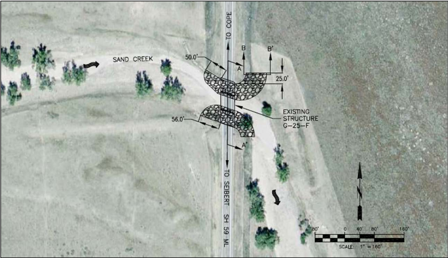
Figure 5. Plan view of Bridge G-25-F with recommended hydraulic scour countermeasure locations
